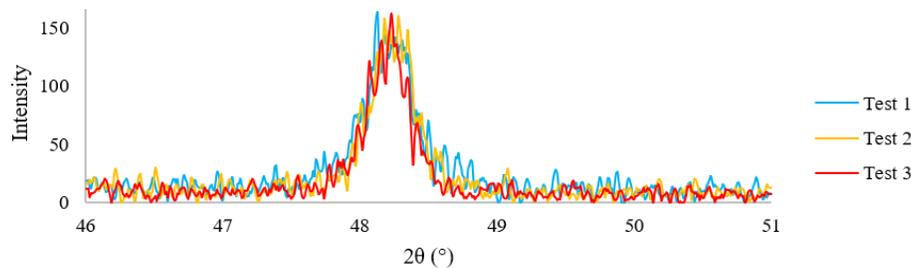
Fig. 2 Grazing incidence ( $5^\circ$ ) XRD line profiles of the WC samples after  $\mu$ -LAM
