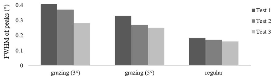
Fig. 3 FWHM of (101) peaks from grazing incidence and regular scans of the WC samples after  $\mu$ -LAM
