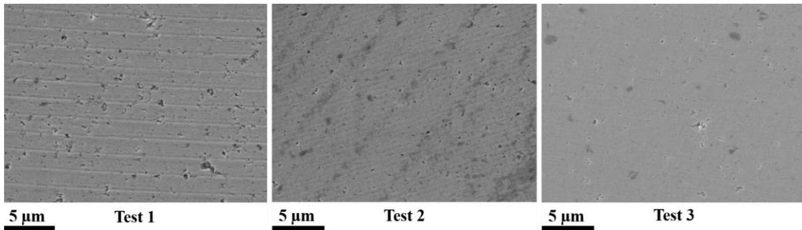
Fig. 1 Secondary electron images of the WC samples after  $\mu$ -LAM
