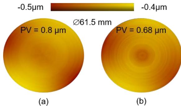
FIGURE 3. Form error measurements for the Si samples; (a) conventional diamond turning (b)  $\mu$ -LAM process
