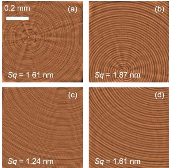
FIGURE 6. SWLI measurements on  $\text{CaF}_2$  sample; (a, b) near center with and without  $\mu$ -LAM respectively (c, d) off-center with and without  $\mu$ -LAM respectively
