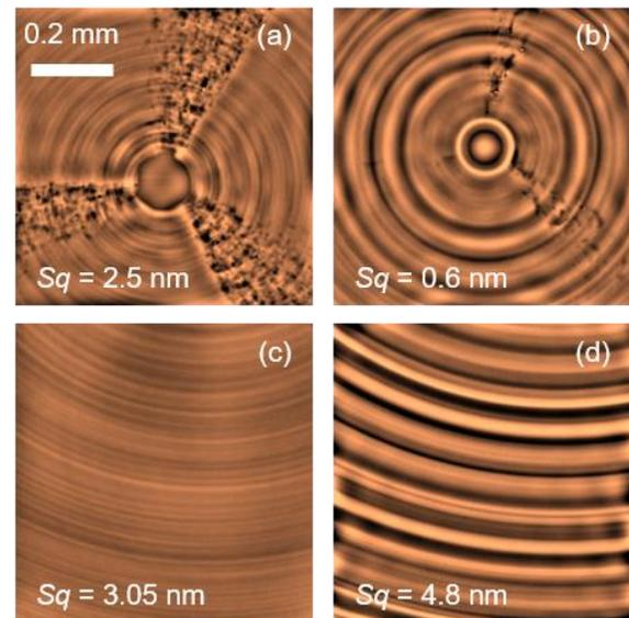
FIGURE 5. SWLI measurements on Si part (a, b) near center with and without  $\mu$ -LAM respectively (c, d) off-center with and without  $\mu$ -LAM respectively
