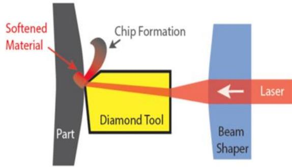
FIGURE 2. The delivery of laser emission at the cutting edge of the diamond tool
