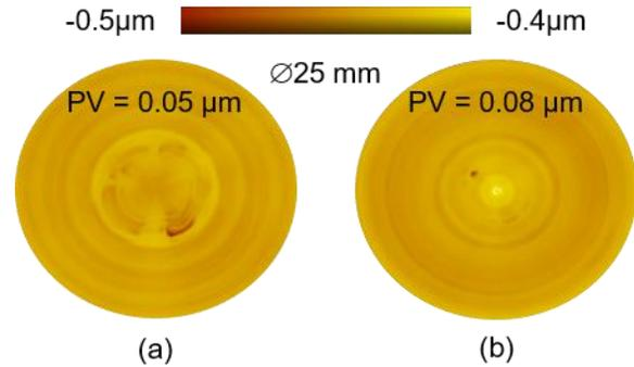
FIGURE 4. Form error measurements for the CaF<sub>2</sub> sample. (a) without  $\mu$ -LAM (b) with  $\mu$ -LAM
