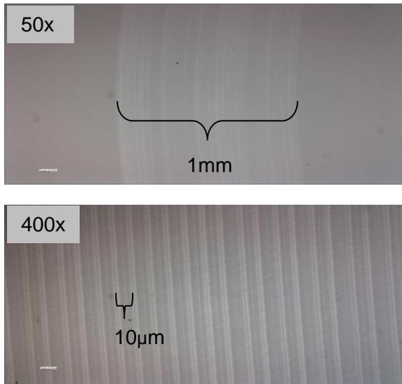
FIGURE 2. Optical microscope images showing the machined region at optimized  $\mu$ -LAM parameters: 10W, 10rpm & 10  $\mu$ m/rev feed.
