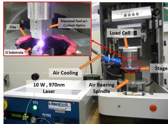
FIGURE 1. Single point  $\mu$ -LAM setup.
