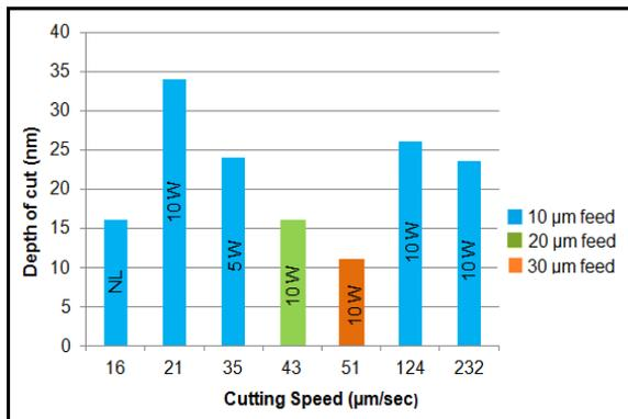
FIGURE 3. Depth of cut and cutting force ratio versus the cutting speed, for varying laser powers and cross feeds.
